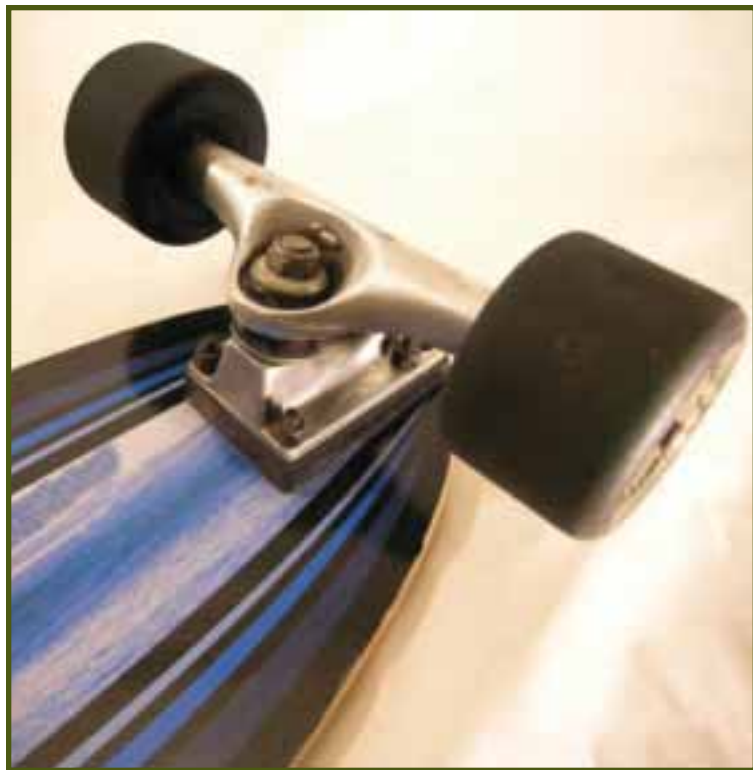
Trucks attach the wheels to a skateboard's deck.
