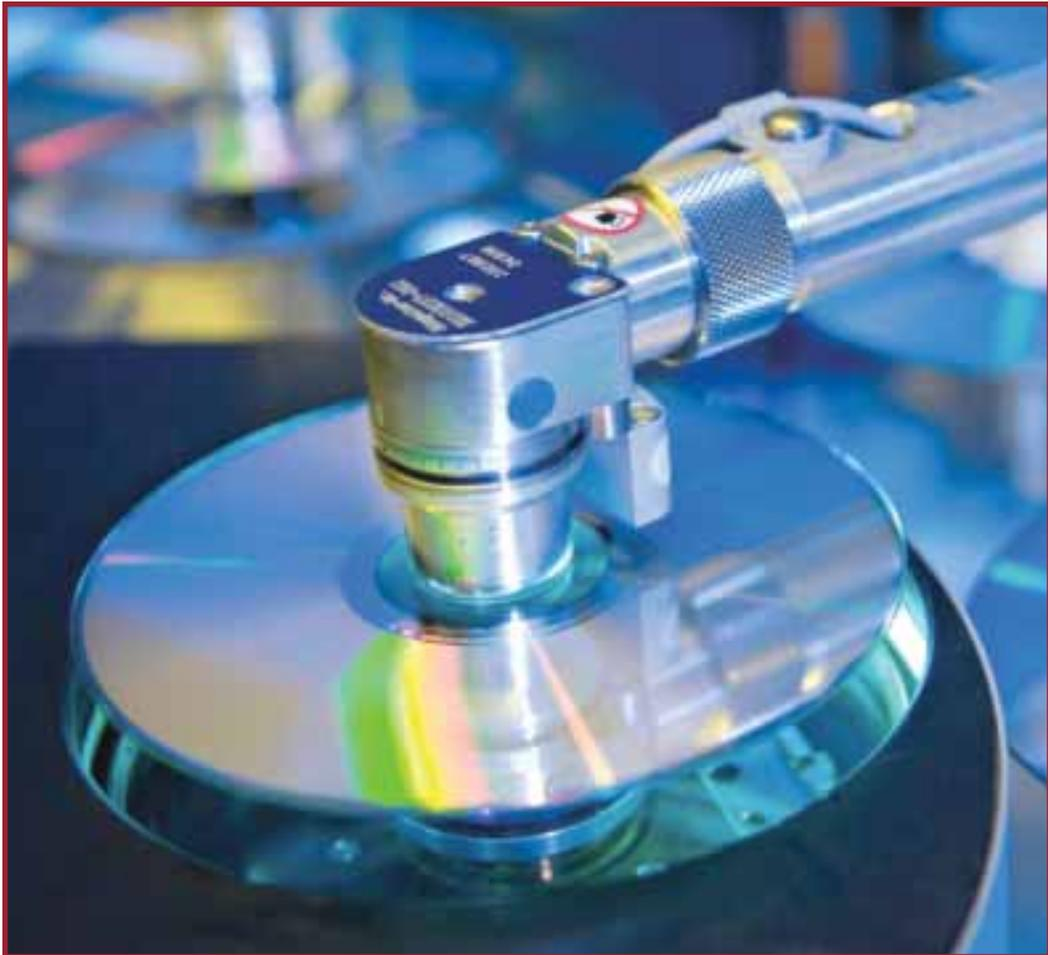
*A reflective coating is applied to a DVD during manufacturing.*
