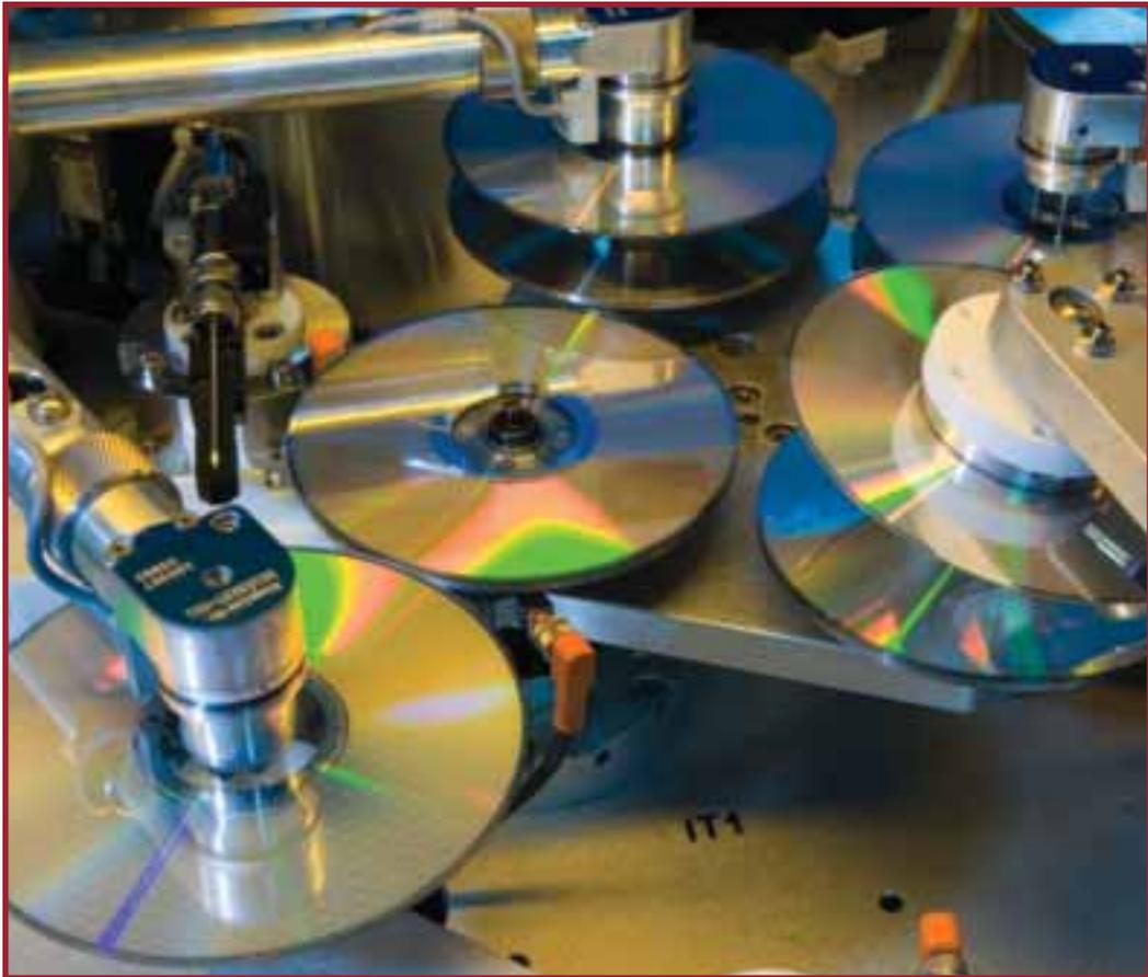
*Dual layers of a DVD are bonded together on an automated production line.*
