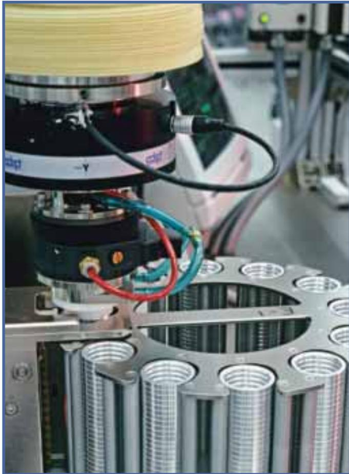
*Part of a computer hard drive is put together by a robot.*
