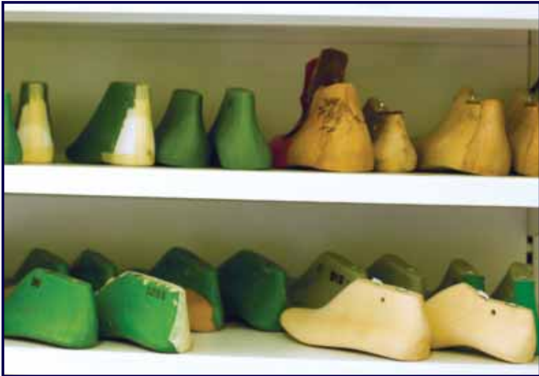
Lasts are shaped like feet and used in the production of all kinds of shoes.
